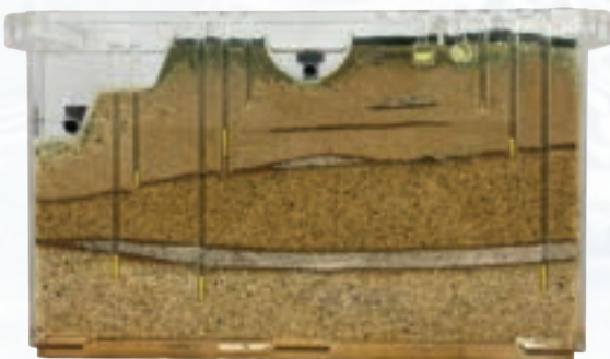
Groundwater model showing a cross-sectional view of different layers of rock, wells, confining layers, and how they interact.
